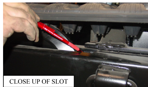
LOCATION OF SLOT FOR CHECKING TRACK TENSION
