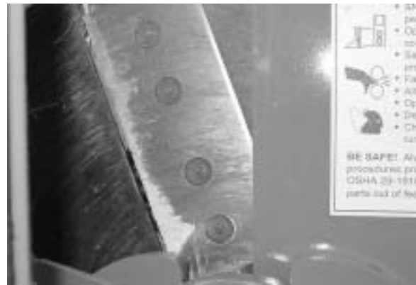
WORN & CHIPPED KNIFE EDGE
