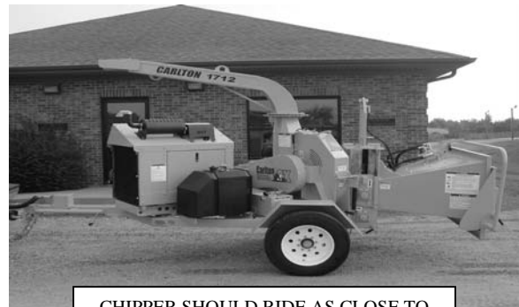
CHIPPER SHOULD RIDE AS CLOSE TO LEVEL AS POSSIBLE WHEN TOWING
