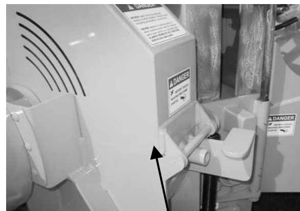
NO GAPS OR OPENINGS
