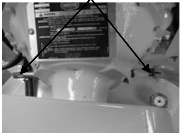
CHECK ENGAGEMENT FORCE AT EITHER END OF THE CROSS-SHAFT
