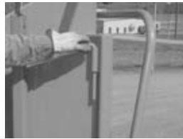
INFEED TRAY LOCK PIN IN STORAGE POSITION (ONE ON EACH SIDE OF CHIPPER)
