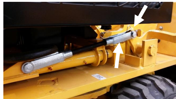
LINKAGE ASSEMBLY ATTACHED TO ENGAGEMENT LEVER. REMOVE YOKE PIN AND ADJUST YOKE.
