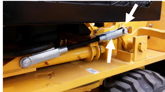
LINKAGE ASSEMBLY ATTACHED TO ENGAGEMENT LEVER. REMOVE YOKE PIN AND ADJUST YOKE.
