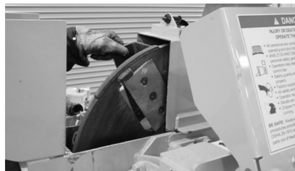
ROTATE CUTTER DISK TO CHECK FOR BINDING
