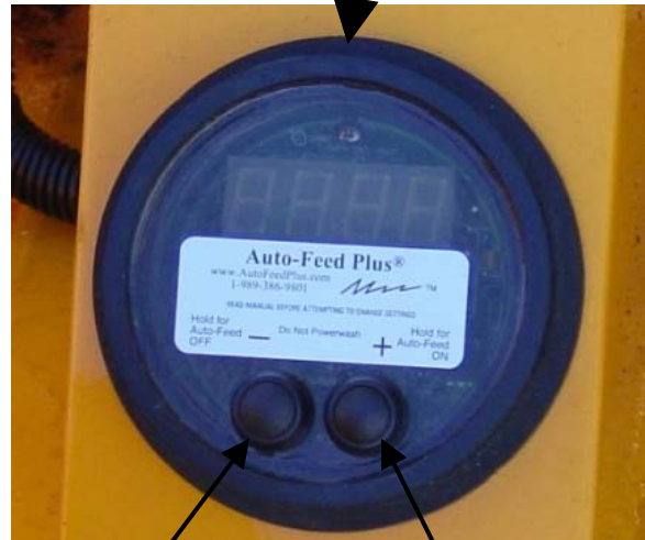
AUTO-FEED OFF (PRESS AND HOLD FOR 4 SECONDS TO TURN OFF)
