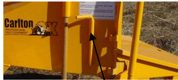
STORED POSITION OF LOCK PINS; ONE ON EACH SIDE OF INFEED CHUTE
