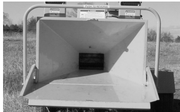
CHECK FOR GAPS OR DENTS AROUND HOOD
