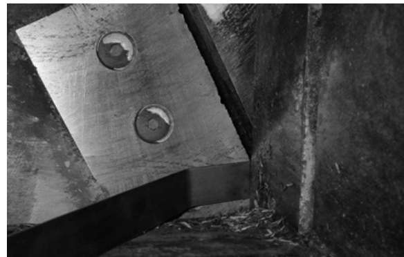
CHECKING KNIFE/ANVIL CLEARANCE
