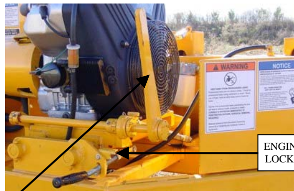
ENGAGEMENT HANDLE SHOULD BE PULLED ALL THE WAY BACK TO THIS POSITION TO ENGAGE THE CUTTER DISK.
