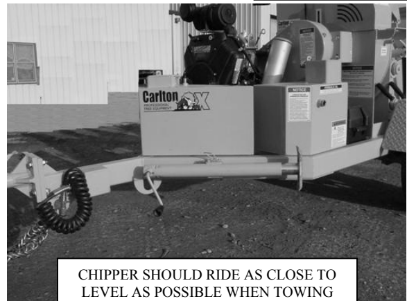
HITCH AVAILABLE IN 2" OR 2 5/16" COUPLER OR 2 1/2" PINTLE RING, PICTURED AT RIGHT.
