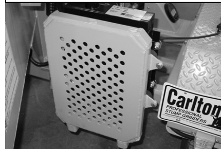
THE OIL COOLER ON THE 6" CHIPPER IS LOCATED ON THE RIGHT SIDE NEAR THE FENDER AS SHOWN HERE
