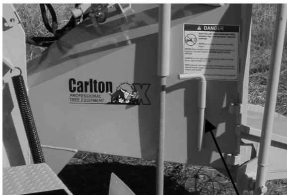
INFEEED TRAY LOCK PIN IN STORAGE POSITION (ONE ON EACH SIDE OF CHIPPER)
