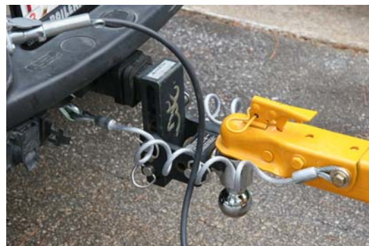
CHIPPER SHOULD RIDE AS CLOSE TO LEVEL AS POSSIBLE WHEN TOWING
