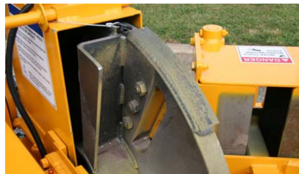
ROTATE CUTTER DISK TO CHECK FOR BINDING
