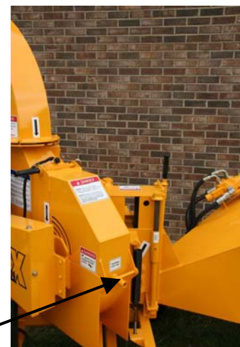
CUTTER DISK LOCK PIN IN LOCKED POSITION
