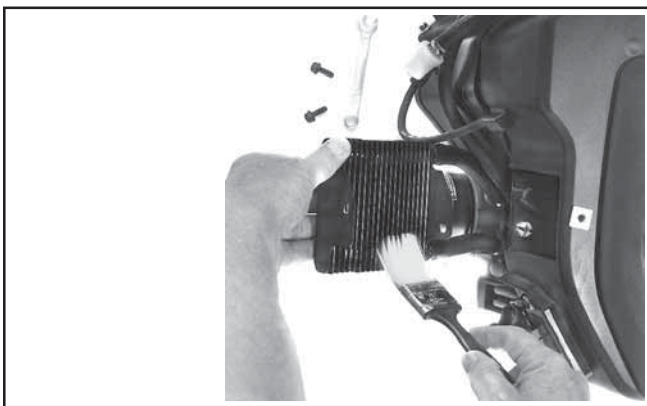
Figure 10. Cleaning Oil Cooler.
