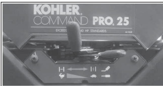
Figure 6. Optional Engine Mounted Throttle and Choke Controls (Carbureted Engines).
