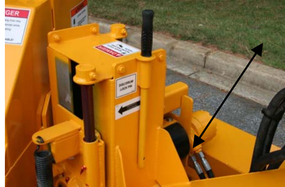
REMOVE YOKE LOCK PIN AND RETURN TO HOLDER
