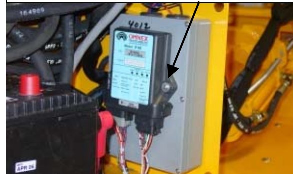
REMOVE THE COVER ON THE REMOTE RECEIVER AND DRILL HOLES TO ATTACH THE RADIO RECEIVER
