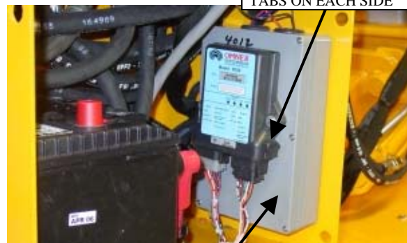
REMOVE THE REMOTE COVER TO ACCESS THE RADIO RECEIVER UNIT
