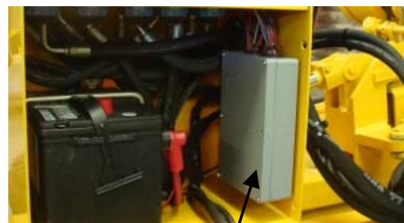
REMOVE THE COVER ON THE REMOTE RECEIVER AND DRILL HOLES TO ATTACH THE RADIO RECEIVER
