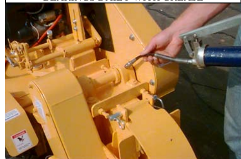
PURGE CUTTER WHEEL AND JACKSHAFT BEARINGS DAILY WITH GREASE
