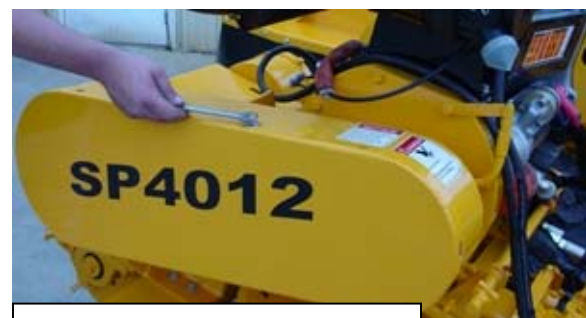
REMOVE V-BELT GUARD COVER AND FOLLOW INSTRUCTIONS FOR REMOVING V-BELT.
