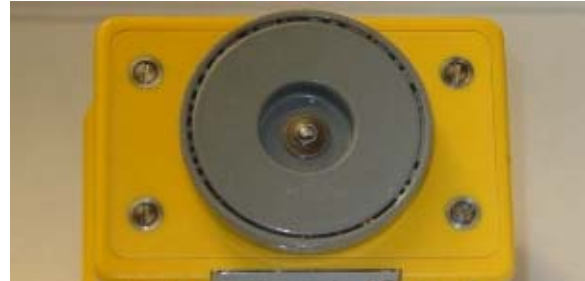
REMOVE THE BACK COVER TO ACCESS THE BATTERIES – THERE ARE 4 SCREWS HOLDING IT IN PLACE. THE BATTERY COMPARTMENT IS LABELED FOR CORRECT BATTERY ORIENTATION.
