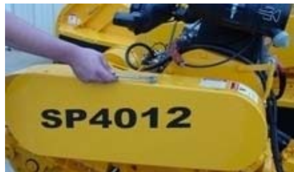
LOOSEN JAM NUT, REMOVE COTTER PIN AND ADJUST CLEVIS TO SHORTEN OR LENGTHEN THE ENGINE SLIDE STOP
