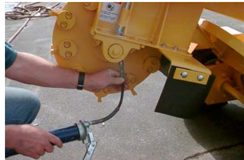
PURGE CUTTER WHEEL AND JACKSHAFT BEARINGS DAILY WITH GREASE
