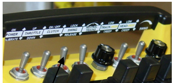
DISENGAGE CLUTCH WITH ENGINE AT IDLE. CLUTCH MUST BE DISENGAGED BEFORE TURNING ENGINE OFF
