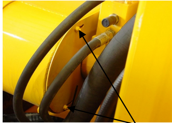
LOOSEN NUTS ON DUST PROTECTION PLATE – 4 PLACES
