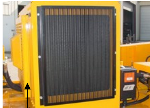
REMOVE BACK ENGINE COVER & CLEAN RADIATOR SCREEN
